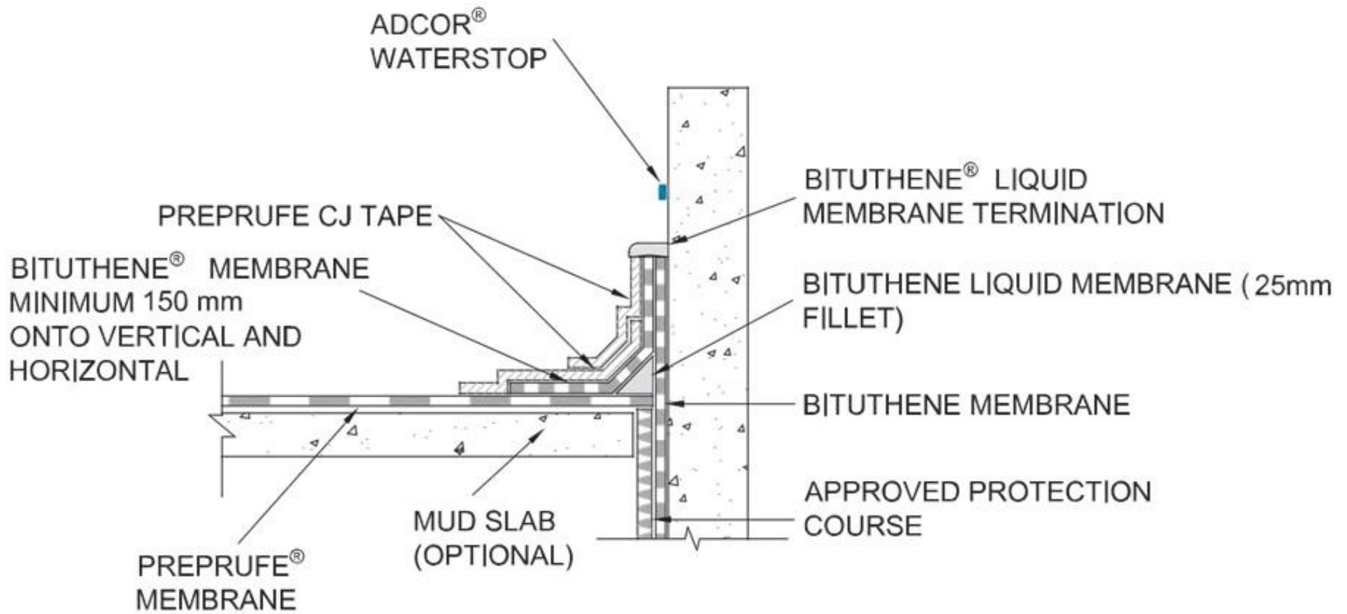
NOTES - IF A MUDSLAB IS NOT USED, THE SUBSTRATE TO ACCEPT THE BITUTHENE LIQUID MEMBRANE MUST BE GROUTED SOLID TO PROVIDE AN ACCEPTABLE SUBSTRATE FOR THE LIQUID MEMBRANE
